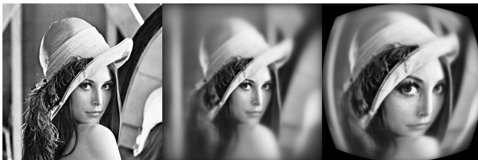
Fig. 8. Space variant photoreceptors subsampling ; from left to right : input picture, space-variant antialiasing filtered picture; Photoreceptors subsampled picture
